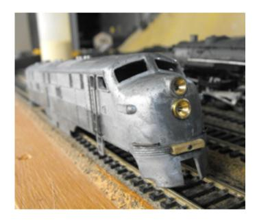
I started rebuilding the 1950's chassis. I removed the brass wheels and replaced them with Northwest Short Line 40" stainless steel wheels. I removed the giant Pittman DC90 motor, this motor was originally designed for O scale models. I replaced it with a Mabuchi RS-387 round can motor, this motor was designed for cordless drill service and has lots of torque.
